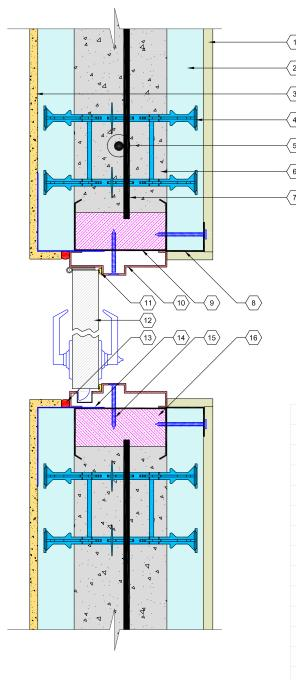
1. INTERIOR WALL FINISH (FASTEN GYPSUM WALLBOARD TO QUAD-LOCK TIE FLANGES)
