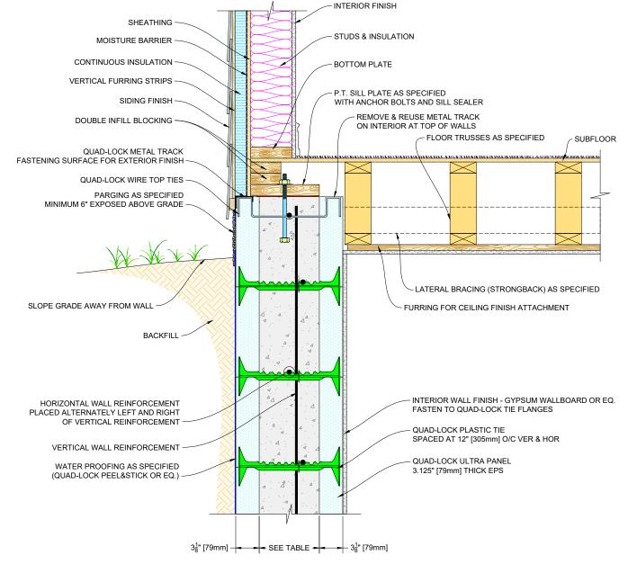
FOR PRESCRIPTIVE DESIGN REFER TO PCA-100 OR IRC SECTION R611 OR APPLICABLE BUILDING CODE FOR SIZING AND OR SPACING OF THE FOLLOWING:
