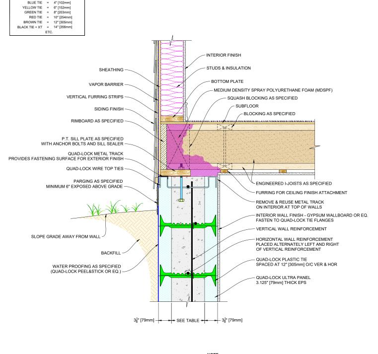
FOR PRESCRIPTIVE DESIGN REFER TO PCA-100 OR IRC SECTION R611 OR APPLICABLE BUILDING CODE FOR SIZING AND OR SPACING OF THE FOLLOWING:
