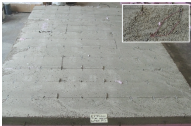
Figure 29. Full height flat-panel ICF with medium-high slump concrete (no mechanical vibration). Note the closeup view of an area with segregation. (IMG13379, IMG13624 [insert])
