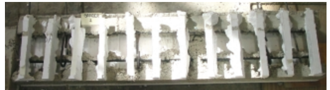
Figure 23. Flat-panel ICF lintel with low slump concrete vibrated with an orbital sander. (IMG13355)
