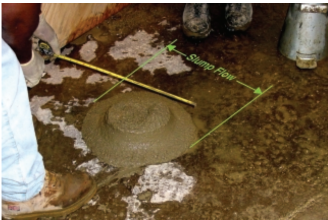
Figure 10. Measurement of slump flow for the SCC. (IMG13342)
