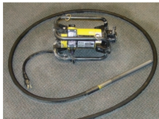
Figure 5. Internal concrete vibrator (disassembled). (IMG13338)
