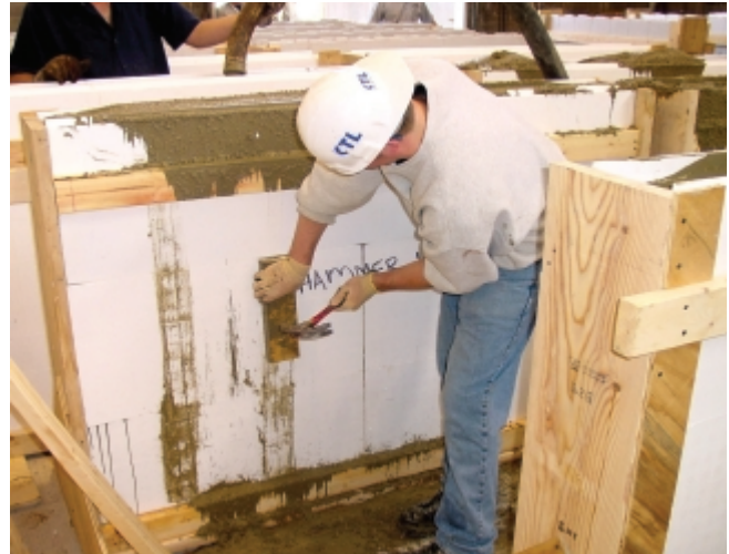
Figure 7. Concrete consolidation using a hammer and block of wood. (IMG13339)
