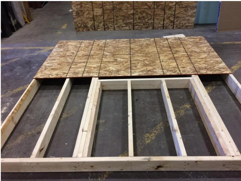
**Construction of the specimen (Specimen #2)**
