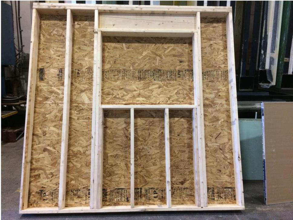
**Construction of the specimen (Specimen #2)**
