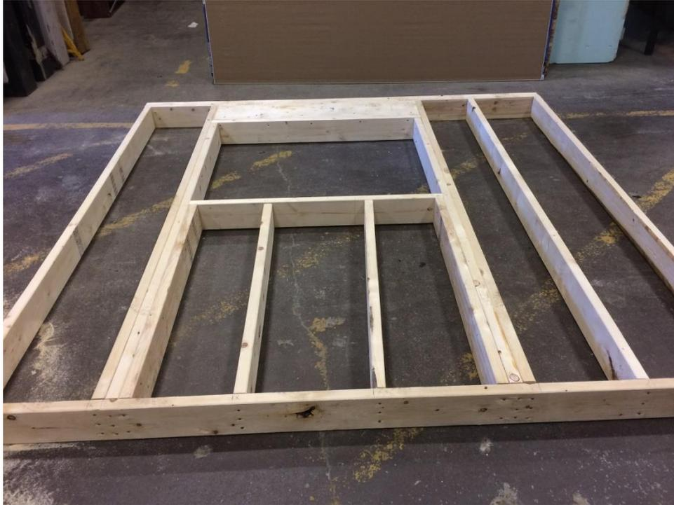
**Construction of the specimen (Specimen #2)**
