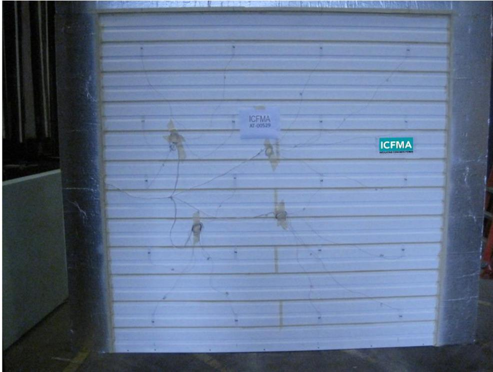
**Interior view of the wall assembly (Specimen #1)**
