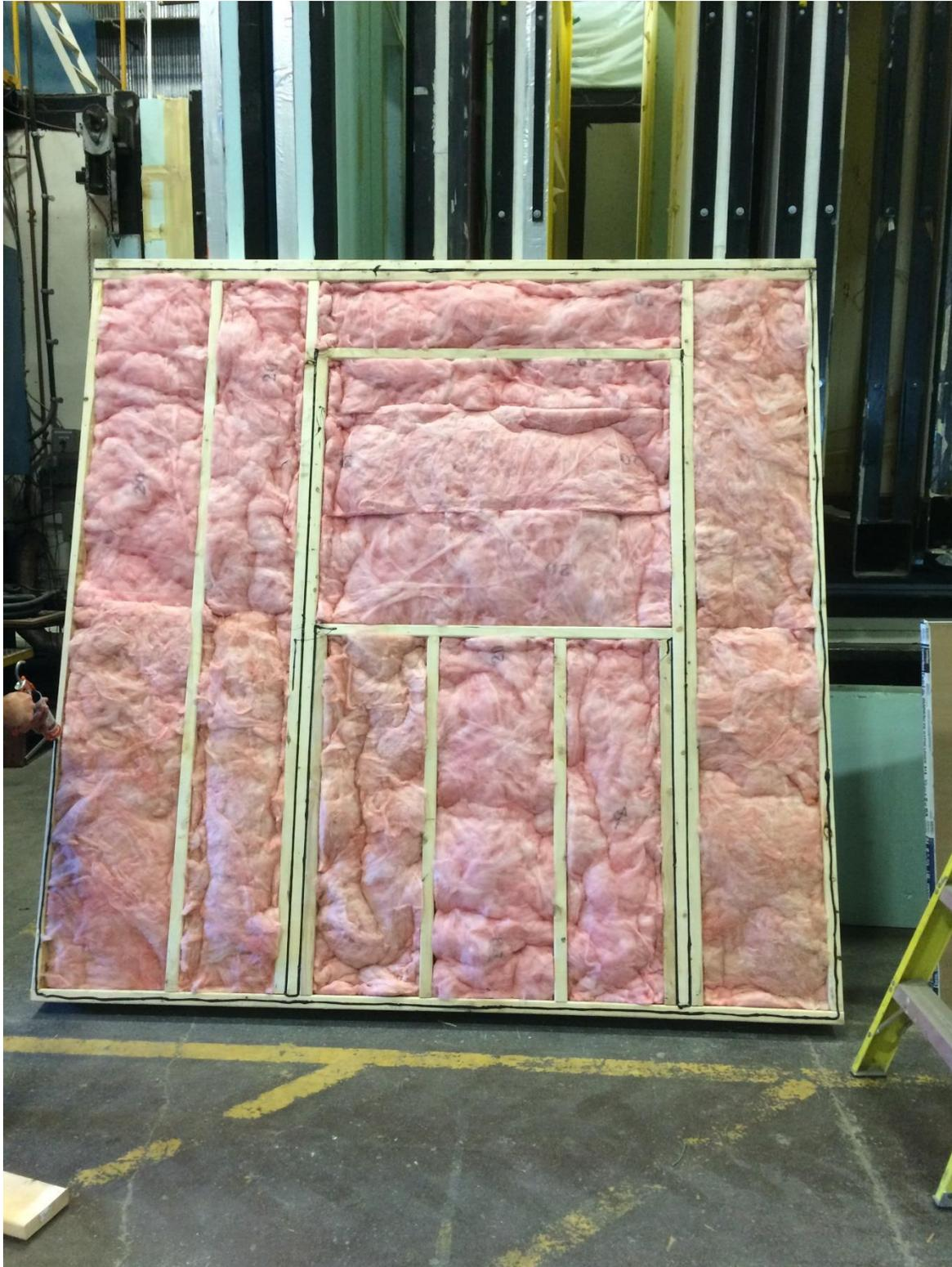
Construction of the specimen (Specimen #2)
