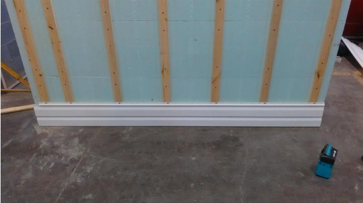
**Construction of the specimen (Specimen #1)**
