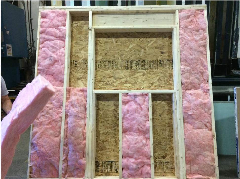
**Construction of the specimen (Specimen #2)**
