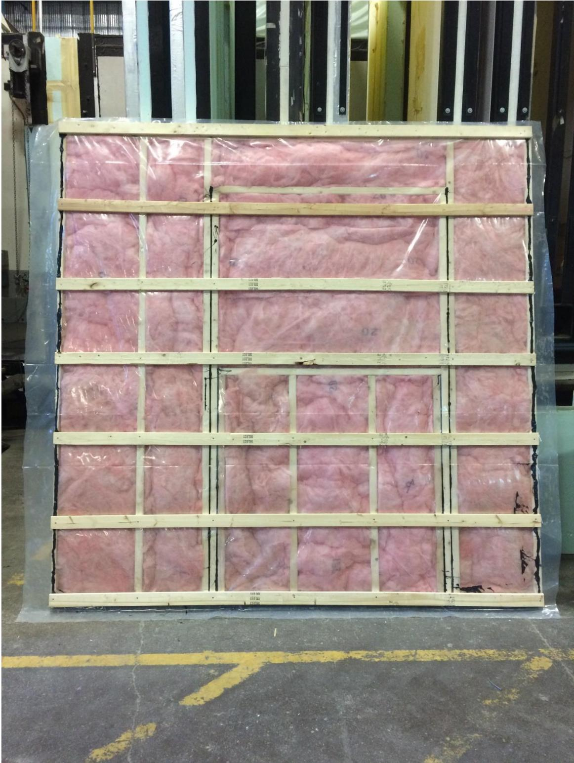
Construction of the specimen (Specimen #2)
