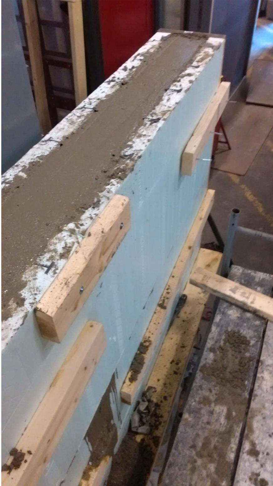
**Construction of the specimen (Specimen #1)**
